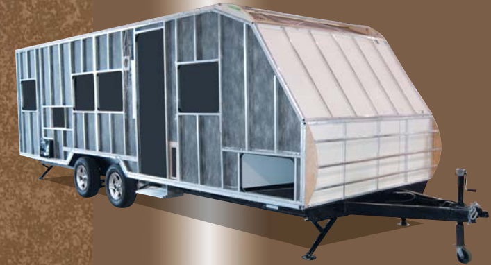
16" OC aluminum studding on all walls and roof
